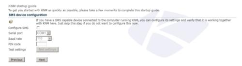
If you have an SMS device connected to a COM port on the **Network Monitor** host you can configure **Network Monitor** to send SMS notifications.
