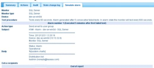
Note: The Simulate alarm feature does not work correctly if the system administrator has disabled all actions.
